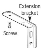
These brackets can be screwed to the top or to the face of a wall or window frame. They should be spaced equidistantly along the width of the blind. Before selecting a fixing point ensure that the brackets will not cover any of the mechanism inside the blind. Brackets should be positioned to one side of any internal fitting.
