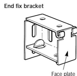
Slide the blind headrail into the brackets ensuring that ALL the slats are hanging below the brackets. Replace the front plates in the end brackets by locating the two projecting lugs into the top of the bracket and swinging the plate downwards to clip into the bottom of the bracket.
