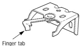
After fixing the brackets pull the finger tabs to the centre of each bracket. Push the blind headrail upwards into the brackets and fold the finger tabs back towards the headrail so that they fit flush with the front of the headrail.
